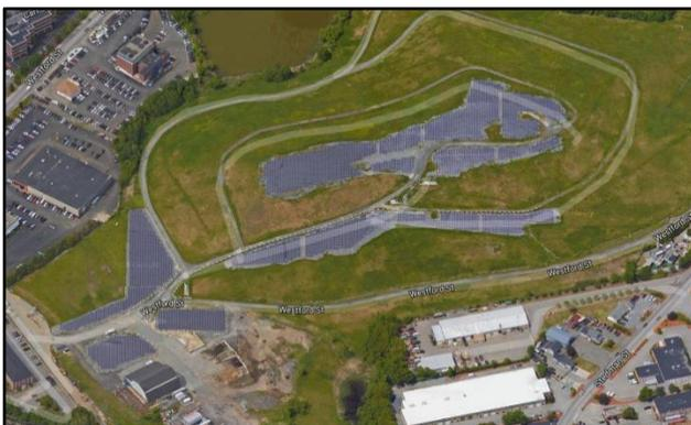
Lowell’s former landfill with its 1.5MW solar array
